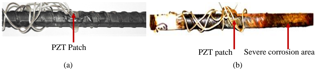
Figure 3.4 Condition of specimens (a) Pristine specimen (b) Corroded specimen
