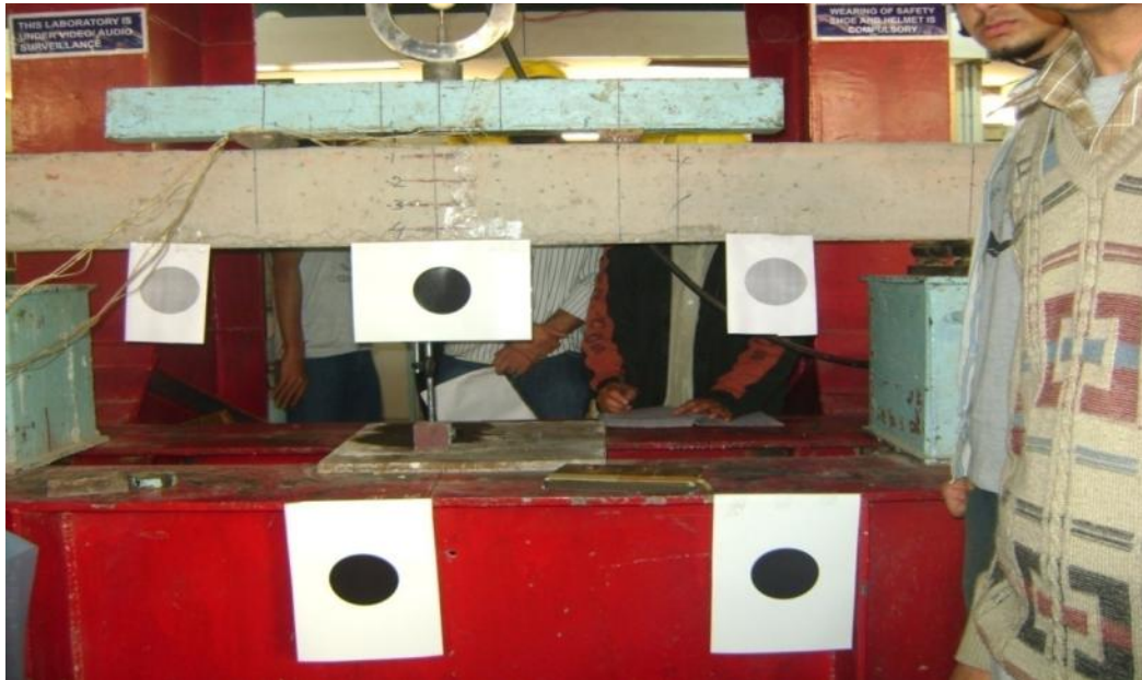
Fig. 7.6 sample picture for reinforced concrete beam photogrammetry experiment
